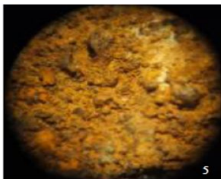
Figure 5: Yellow-colored and furuncles corrosions on the surface of object number 2 with magnification of 40 x.
