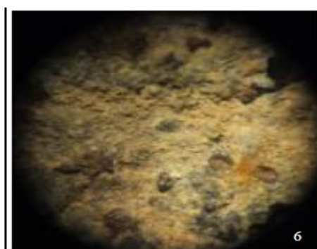
Figure 6: Dust and minerals deposits on the surface of object number 1 with magnification of 40 x.
